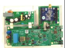
Test Tool PLC+RF Tester Modem PLC Tester Modem RF Certification Test Procedures
