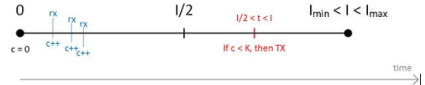
Figure 1 : General principle of the application of the Trickle algorithm over interval I
