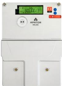
**Apator NILEE Smart Energy Meter** – 1-phase and 3-phase meters with **energy management** functionality (realised by additional user Edge applications), rich connectivity (PRIME 1.3.6, PRIME 1.4, G3-PLC standards, LTE, Wi-Fi), USB stack and optional PLC data concentrator function.
