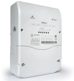
**Data Concentrator Unit - 8K devices** for Energa-Operator S.A., gather data from 2M smart meters in power grid (the largest implementation in Poland). Devices with TCP/IP communication and several security protocols used (IPSEC, 802.1X, TLS), support PRIME 1.3.6, PRIME 1.4 PLC standards.
